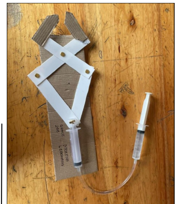
As part of their Design Technology, Grade 7 made simple mechanisms that move by means of hydraulics.
